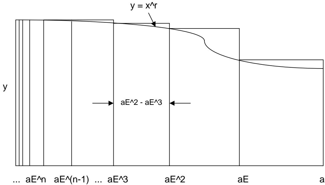
Set  $E < 1$  and divide interval [0 to a] as shown above. Note that there are an infinite number of intervals shown.
