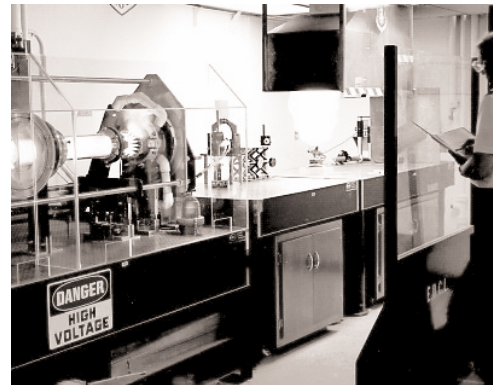
Figure 5. CO2 Laser Used to Study the Energy Incident on the Effects of Radiation on Materials (Reference 9)
