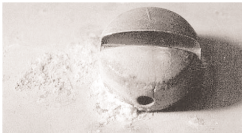
Figure 6. Galvanic Corrosion between a Stainless Steel Screw and Aluminum (Reference 10)
