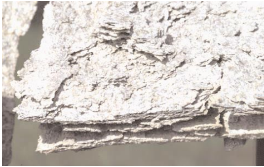
Figure 8. Exfoliation of an Aluminum Alloy in a Marine Environment
